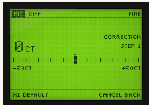
FINE VIEW A pitch block's correction parameter at its default, 0 cents, range -50 to +50.
