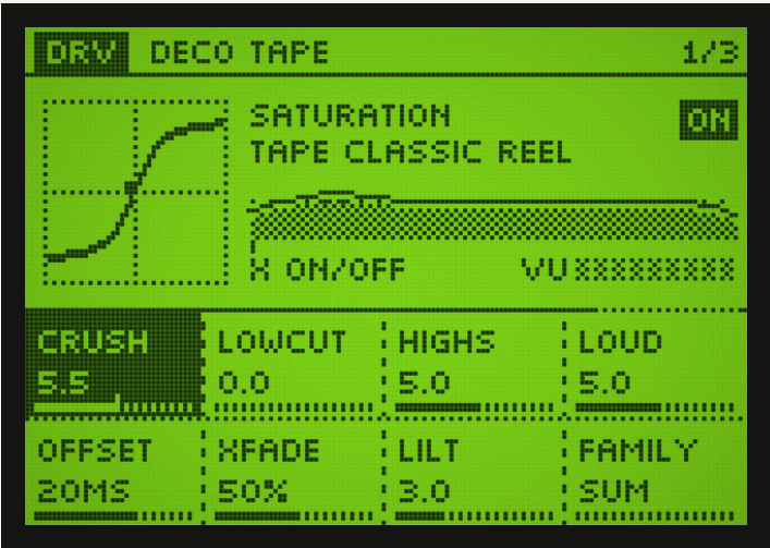
EDITOR A drive block on page 1 of 3, with CRUSH selected. The VU meter and curve follow your playing.
